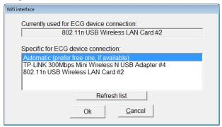
In those cases, where **only one interface** is available in the system and internet access if required for Cardiax (e.g. mailing) or for other activity a solution is provided to allocate the WiFi interface for direct connection to the ECG device **only for the time of recording**. This can be achieved by checking the 'Only establish direct WiFi connection while recording' option.
